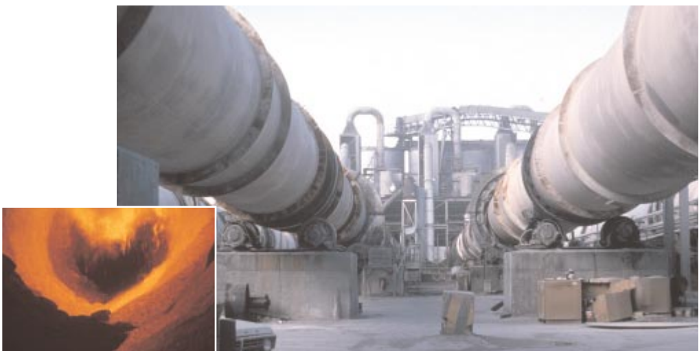
Figure 3.3.1. Rotary kilns in operation at a cement plant.
