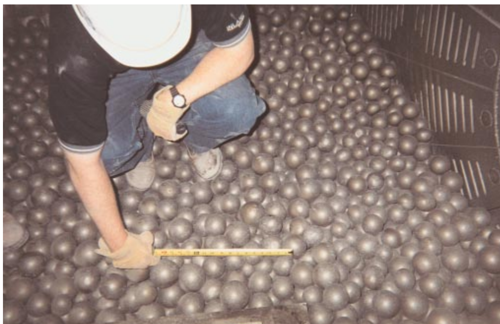
Figure 4.1.6. Grinding balls in the first compartment of the ball mill.
