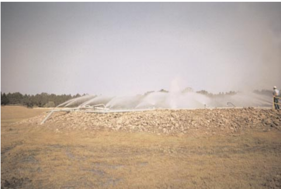
Figure 6.4.1. Water processing pond using spray nozzles at cement plant.
