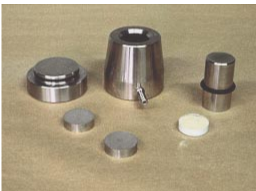
Figure 8.1.6. Disassembled briquette press and aluminum samples caps. Pellet producing the finished surface of the briquette should be highly polished and free from scratches.
