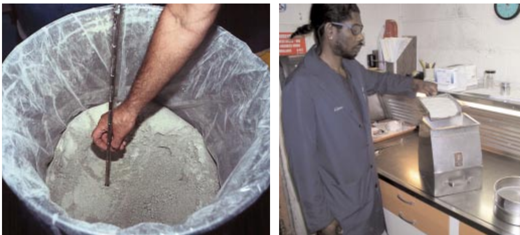
Figure 8.1.2. Use of a sample thief is recommended when sampling from a bulk container. Open the thief lengthwise on a clean paper to view the sample throughout its depth. A riffle-splitter is used to reduce samples to laboratory size.
