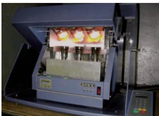
Figure 8.1.7. A three place Claisse® flame unit in operation. Temperature, time, and cooling are all important for fabricating good quality fusion glass beads.
