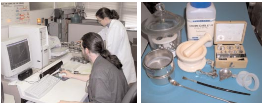
Figure 8.1.1. (left) Modern X-ray spectrometer use in cement analysis. (right) Specimen preparation equipment for cement and related materials include borate flux, mortar and pestle weighing dish, sieves, dessicator and the resulting specimen ready for analysis including loose powder cup, pressed powder and fused bead.
